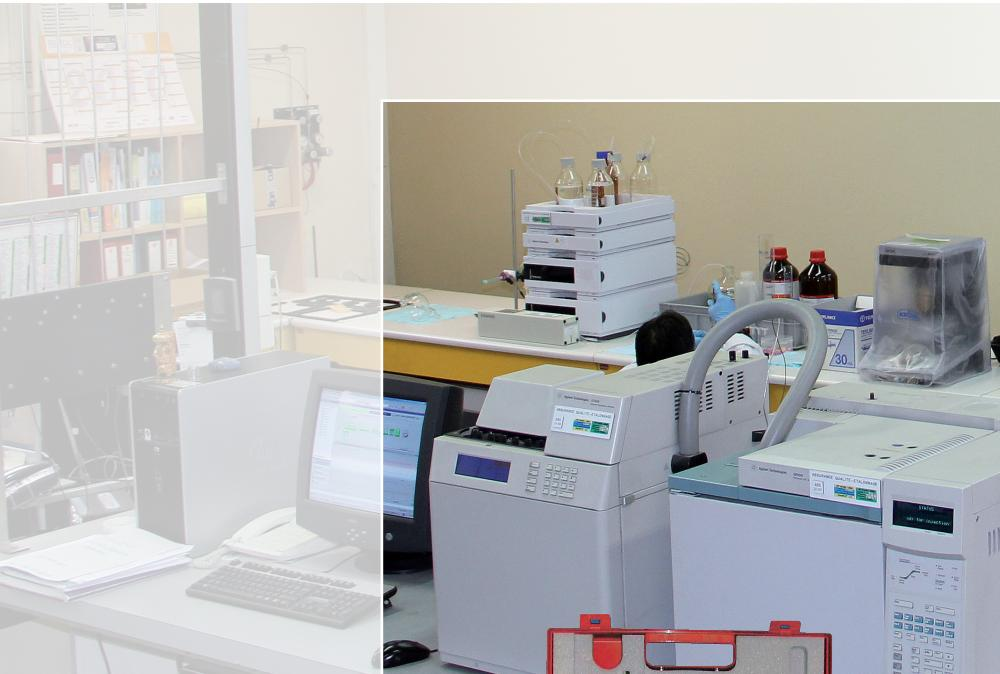
**Chromatography of dissolved gas**, taking oil samples and carrying out a chromatographic analysis in gaseous phase of the dissolved gas content:
